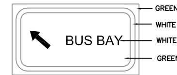
BUS BAY SIGN I-7
